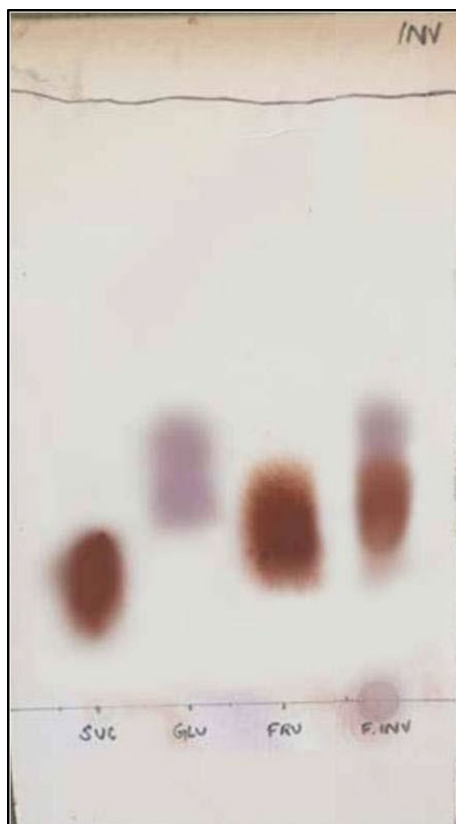
Fig. 3 Thin layer chromatogram of Aspergillus sojae \beta -D-fructofuranosidase loaded with the standards. Lane 1: D-sucrose, lane 2: D-glucose, lane 3: D-fructose, lane 4: enzyme hydrolysate spotted after an overnight incubation at 37 °C, representing D-glucose and D-fructose released from the disaccharide
