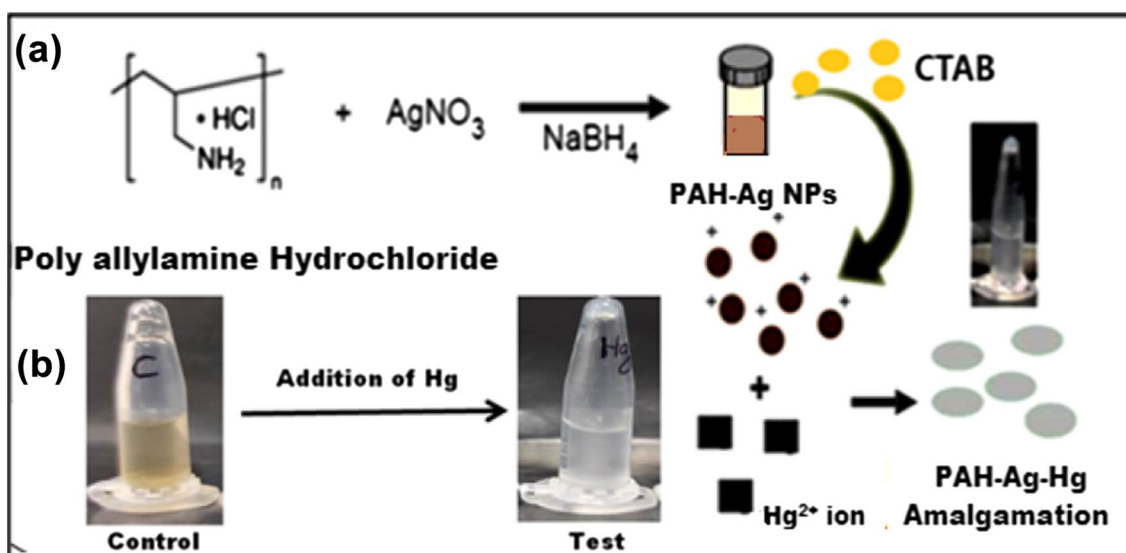
Fig. 1 a Pictorial representation of amalgam formation of PAH–Ag nanoparticles when reacted with \text{Hg}^{2+} ions. b Inset shows PAH–Ag in dispersed phase is yellow in color becomes colorless when mercury is added to it
