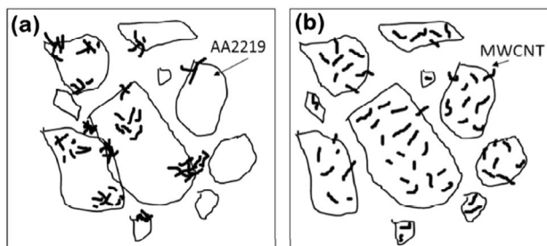
Fig. 10 Schematic representation of MWCNT in AA 2219 after a ball milling for 4 h, b premixing followed by ball milling for 4 h (Thomas et al. 2019b)
