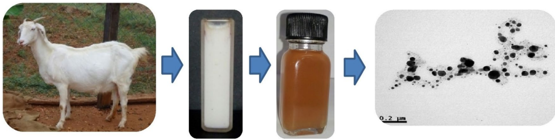
Fig. 1 Process of goat milk mediated AgNPs synthesis
