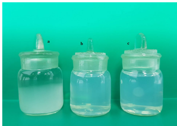
Fig. 5 Photographs of vials with nanocellulose suspensions prepared after 24 h of TEMPO-mediated oxidation of ORP: a without ultrasonic treatment; b after ultrasonic treatment, and c after 4 months of storage
