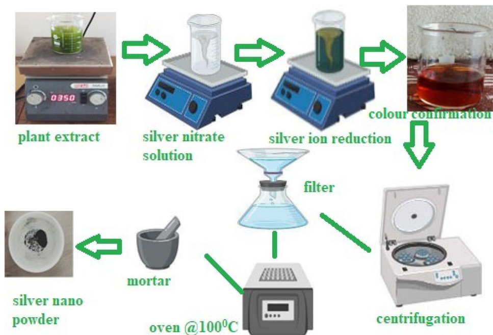
Scheme 1 The reaction between plant extract ( Cyperus pangorei ) versus silver nitrate. A representation of the Ag NPs synthesis process
