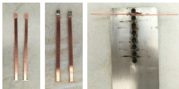
Fig. 1 Preparation of the hybrid solder joints
