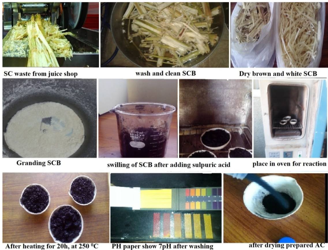
Fig. 1 Grinding process of dry sugarcane bursesses
