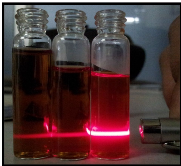
Fig. 10 Laser light path traversing through Ag-NPs colloids
