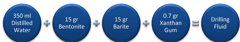
Fig. 4 Drilling fluid preparation
