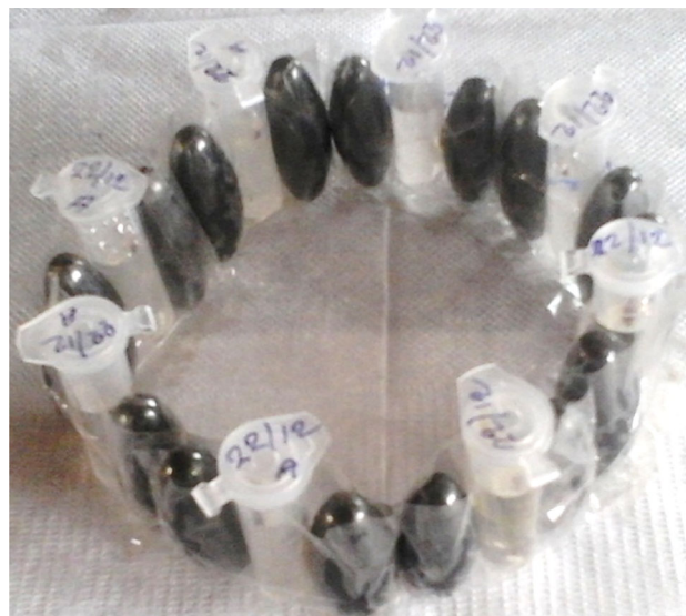
Fig. 1 Precursor ionic molecular solution kept in the magnetic field for the synthesis of SPIONs
