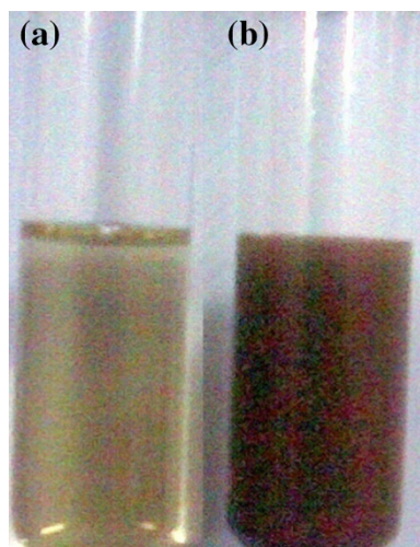
Fig. 1 a Plant extract, b plant extract with silver nitrate (SNPs) the color change of stem bark extract of C. religiosum
