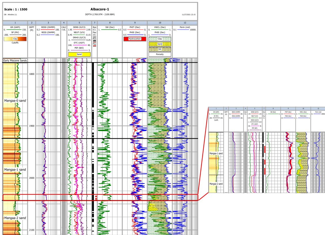
Fig. 4 Litho-saturation cross-plots of the Mangaa Formation showing the porosity, water saturation and the shale volume in addition to the reservoir and pay zones of the Albacore-1 well
