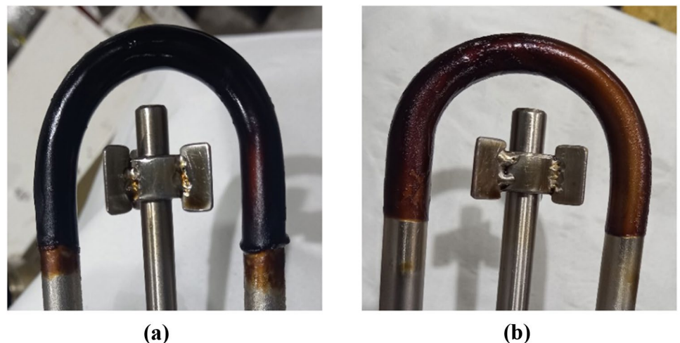
Fig. 4 Cold finger temperature effect on the deposition of wax, a 5 °C and b 10 °C
