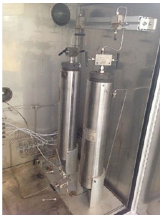
Fig. 2 Static ageing experiment set-up. The experiment was conducted for 45 days using synthetic brine created to mimic the real formation brine of the carbonate reservoir being studied
