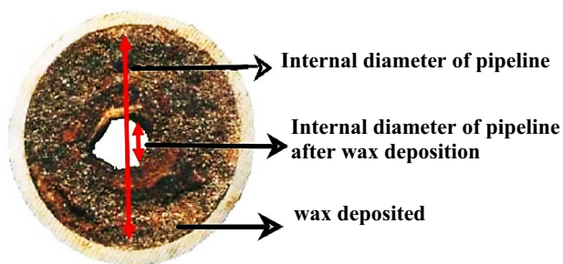
Fig. 1 Plugged pipeline. Adapted from “A unified perspective on the phase behaviour of petroleum fluids” Source: (Mansoori 2009)
