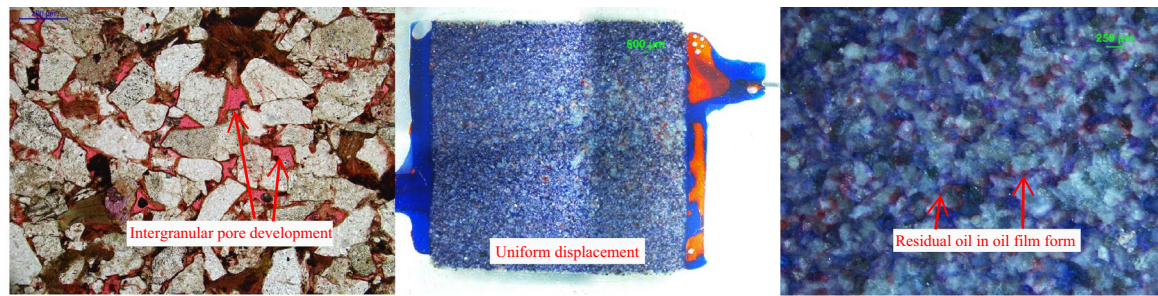
a. H393, intergranular pore development, uniform displacement, the final oil displacement efficiency of 61.78 %
