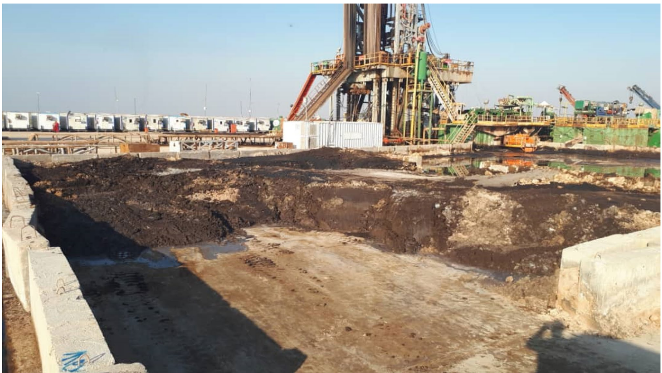
Fig. 2 Returned lubricant mixed with soil in the waste pool without having any standard cover
