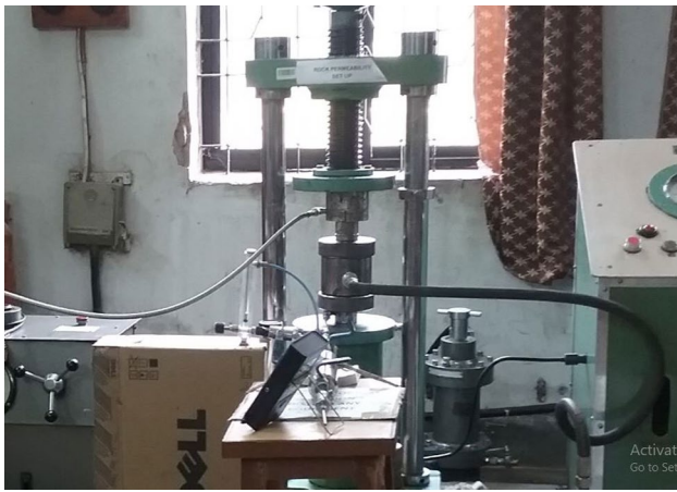
Fig. 4 Experimental set-up for coal gas permeability
