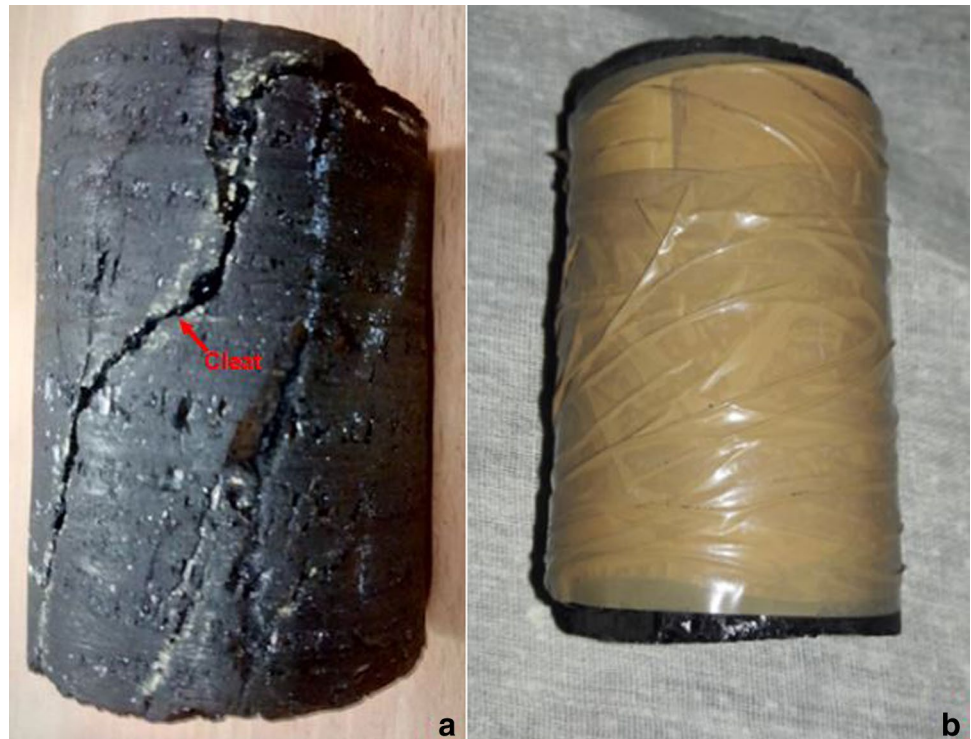
Fig. 2 a Unrapped sample showing cleats, b wrapped sample for permeability testing
