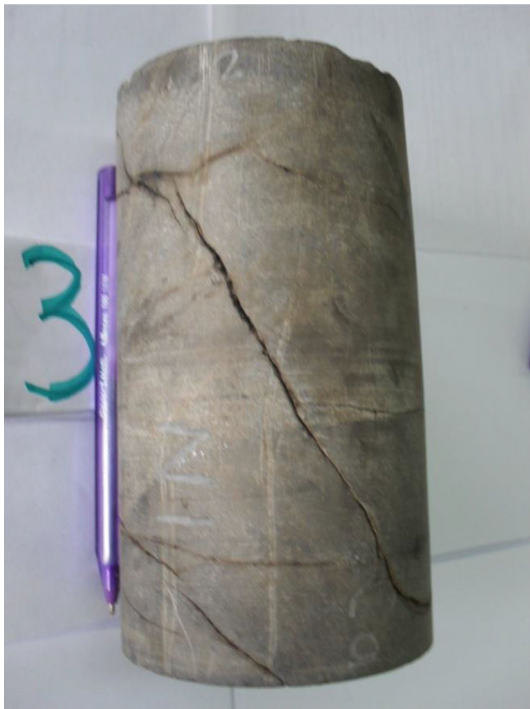
Fig. 3 Tectonic fractures in a core of NFTR
