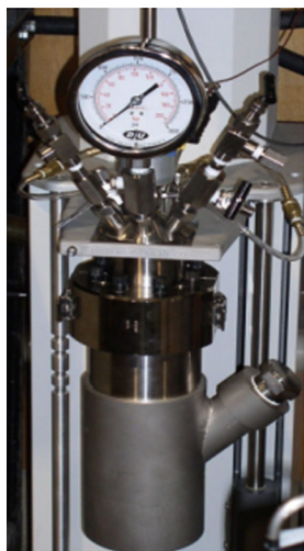
Fig. 3 Traditional Parr autoclave model 4547
