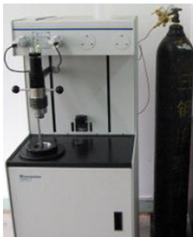
Fig. 3 Micro-Meritics automatic mercury intrusion apparatus (Auto-Pore IV)
