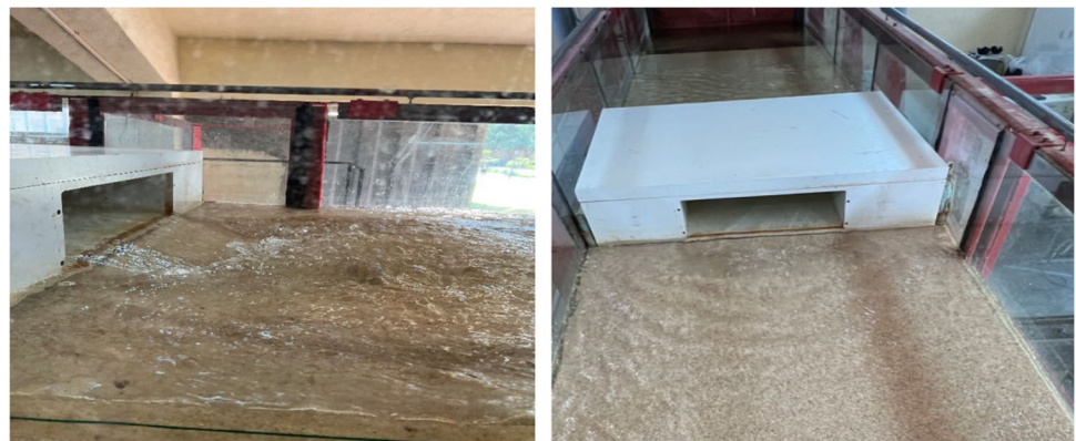
Fig. 8 Culvert output jet at level Z=0.067b
