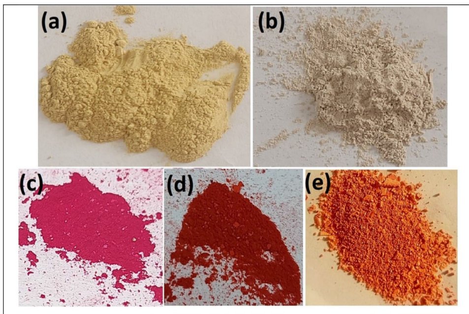
Fig. 1 Digital photographs of a Bt, b Bt@CTAB, c Bt@CTAB-E122, d Bt@CTAB-E124, e Bt@CTAB-E110
