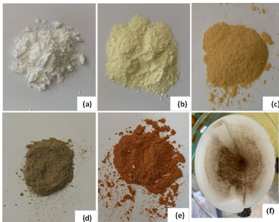
Fig. 11 Optical images of a Native cellulose powder, b DAC oxidized cellulose, c DAC@GuTSC, d DAC@GuTSC-Cu, e DAC@GuTSC-Hg and f DAC@GuTSC-Pb
