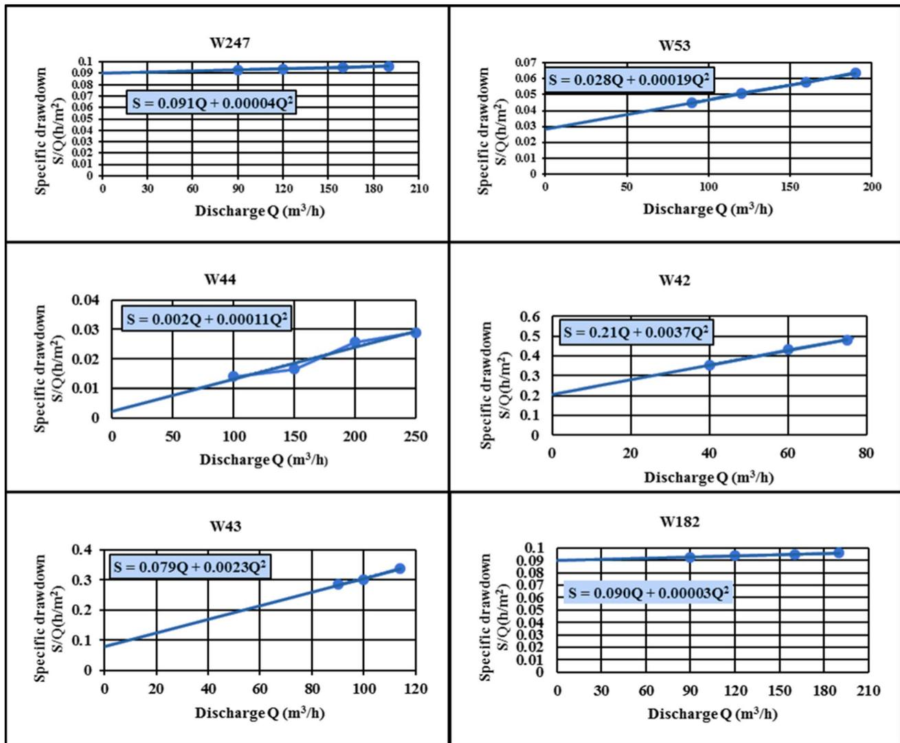
Fig. 11 Step test diagrams from pumping test for the Eocene aquifer, West–West Minya, Egypt
