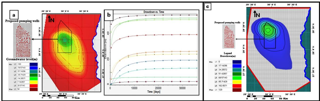
Fig. 17 Model results of the second simulated scenario: a hydraulic head distribution, b drawdown versus time, and c drawdown distribution
