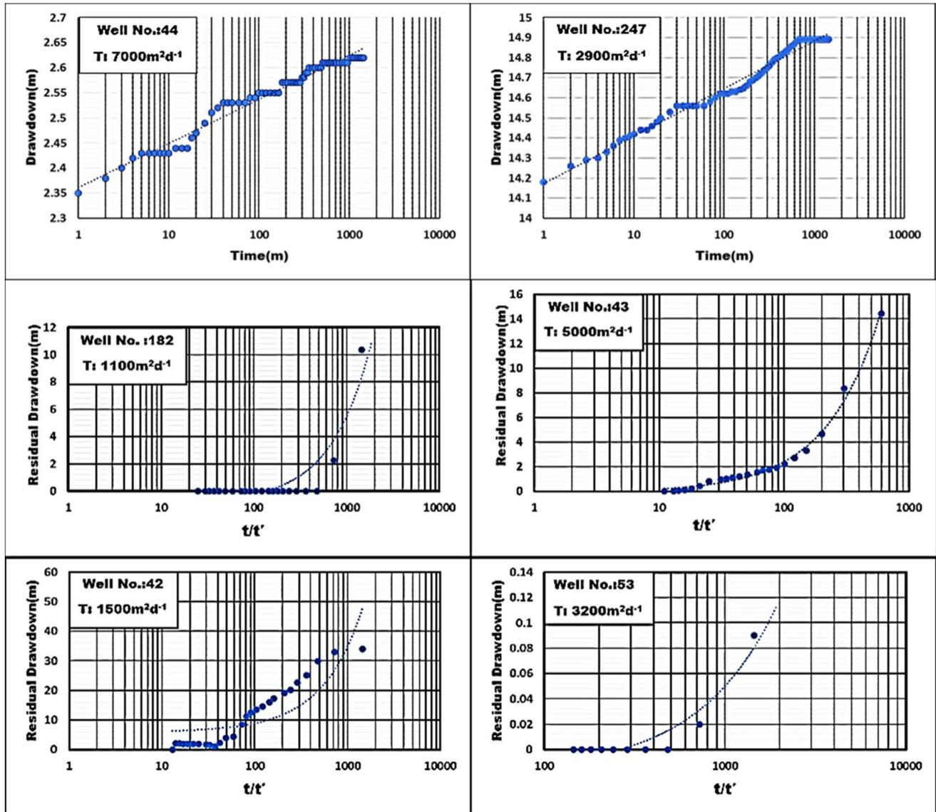
Fig. 12 Constructed curves of constant discharge pumping and recovery tests for the Eocene aquifer, West–West Minya, Egypt
