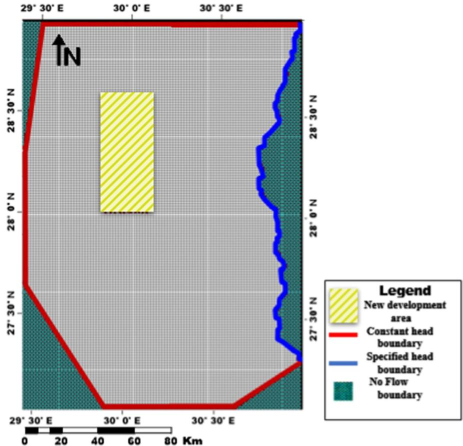
**Fig. 10** Initial distribution head in the modeled area
