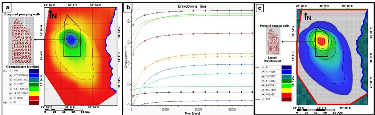
**Fig. 16** Model results of the first simulated scenario: **a** hydraulic head distribution, **b** drawdown versus time and **c** drawdown distribution
