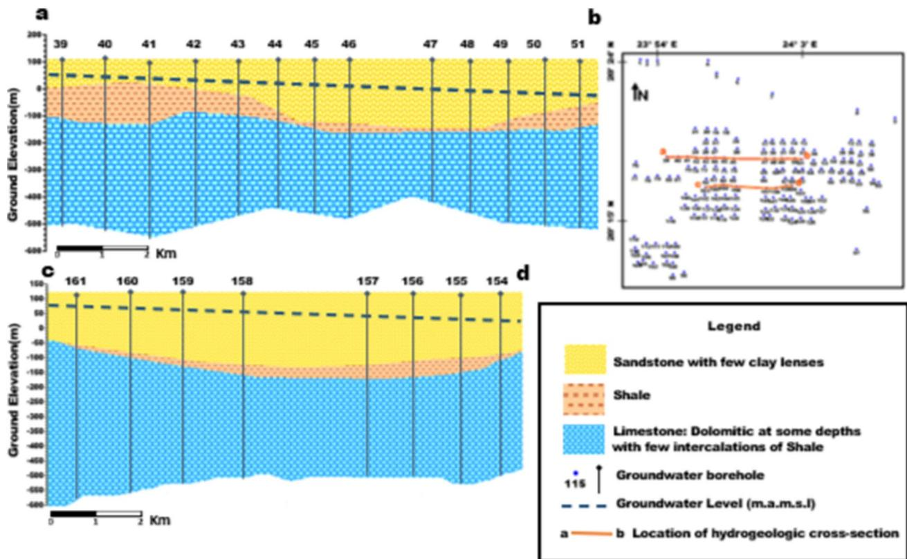
Fig. 5 Hydro-stratigraphic cross sections in the new development area
