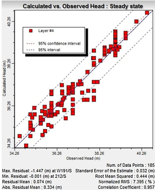
**Fig. 14** Scatter plot of observed versus calculated heads in the steady-state calibration
