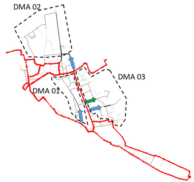
Fig. 8 Directions of DMA water supply (blue arrows). The transmission segments were marked in red, whereas the new pipe supplying DMA 03 was marked as a green arrow
