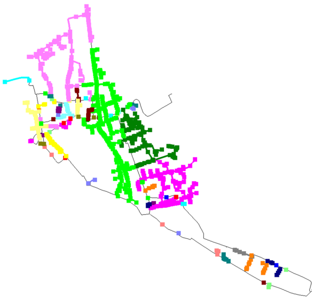
Fig. 4 The analyzed zone divided into DMAs generated by means of the WaterGEMS software (DMA-Tool)
