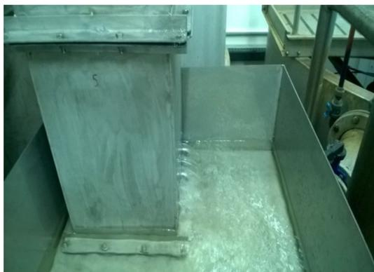
**Fig. 3** Last segment of the aerator with aerated water outflow
