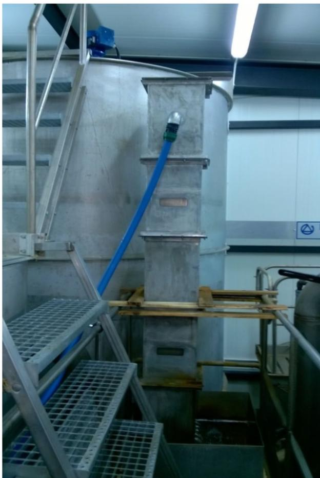
**Fig. 2** Aerator for water aeration
