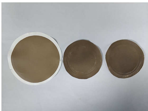
Fig. 10 Digital photographs of c-GO-PEI membranes before (left) and after test with 6.36 ppb (center) and 9.4 ppb (right) Hg-containing wastewaters that washed with DI water
