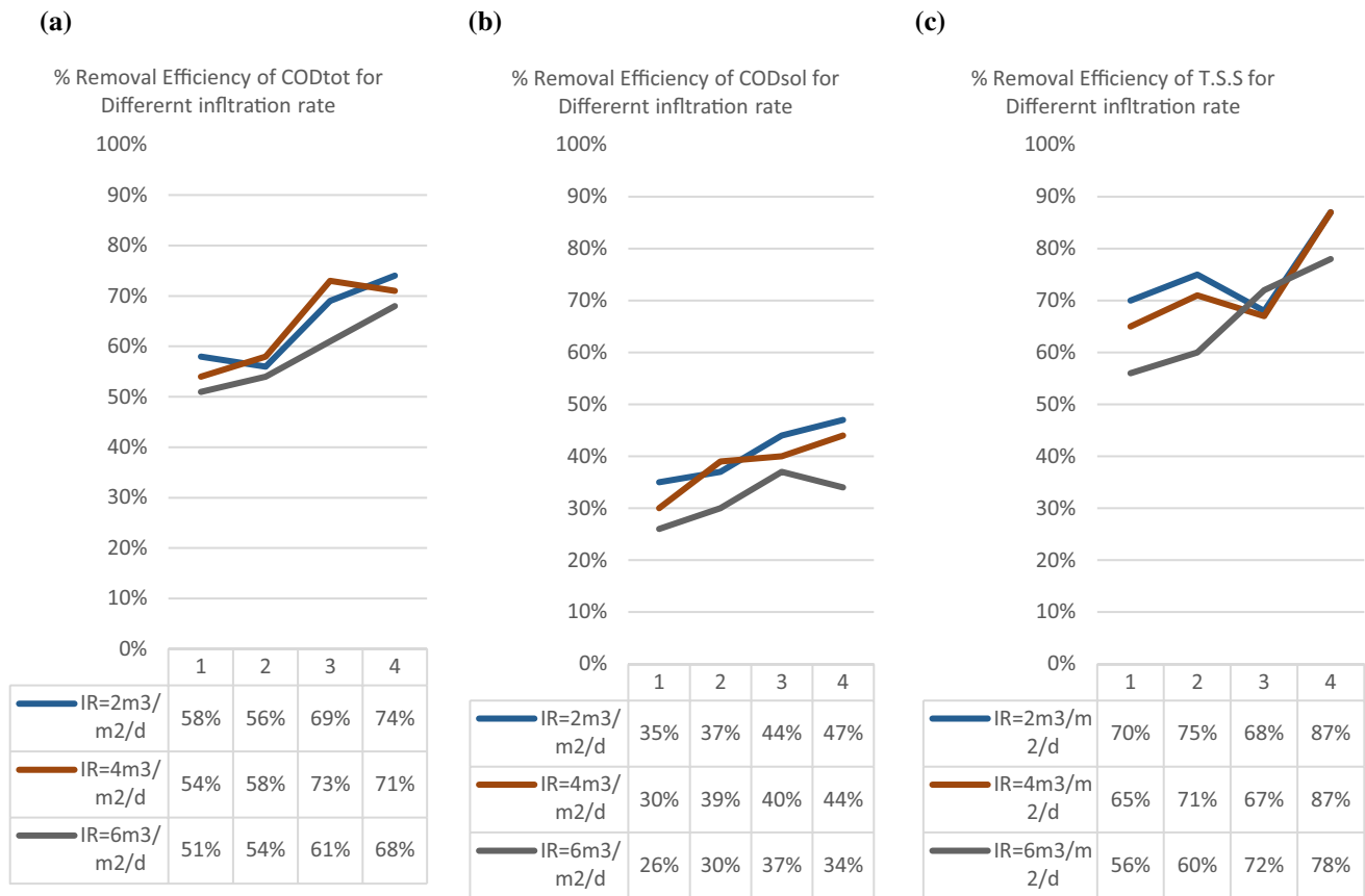
Fig. 13 Results obtained from run (3), a) %R.E. of COD tot for different I.R, b) %R.E. of COD sol for different I.R, c) %R.E. of TSS for different I.R
