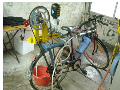
Fig. 16 Pedal powered UF system. Photo: Ramprasad V
