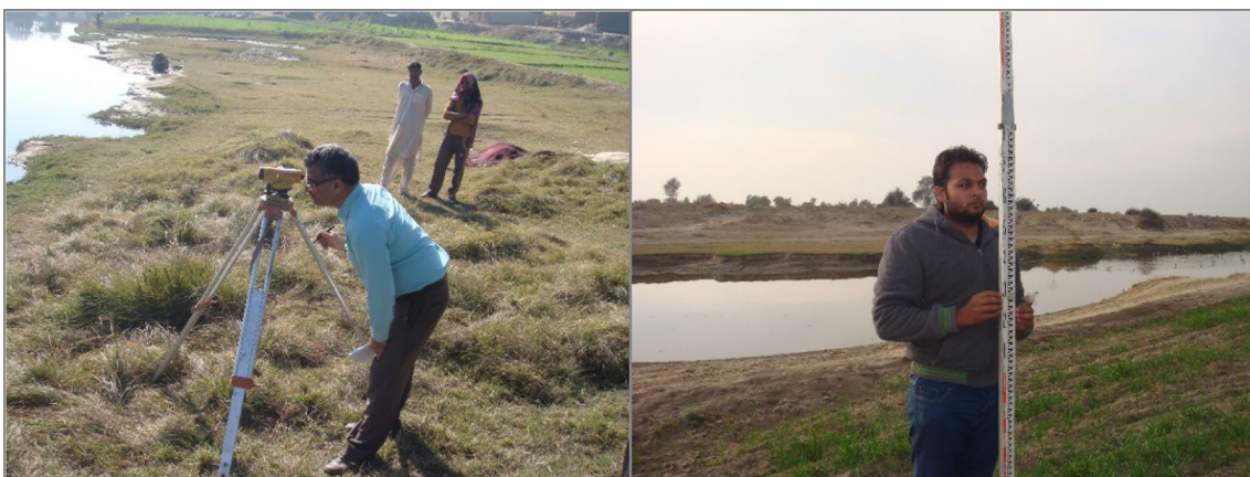
Fig. 5 Leveling survey being carried out (near Muhammad Pura village)
