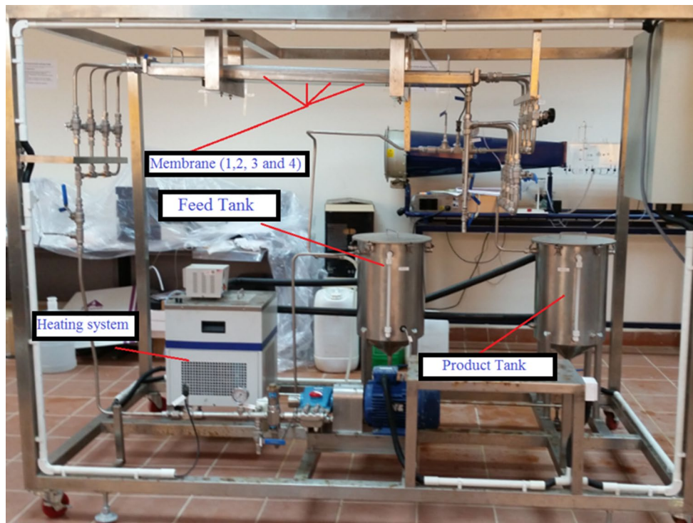
Fig. 4 The membrane filtration test unit; Model: TR 14
