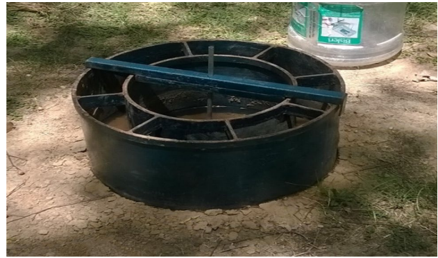
Fig. 2 Double ring Infiltrimeter
