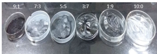
Fig. 2 Prepared membranes of chitosan-modified biochar with varying proportions of biochar:chitosan
