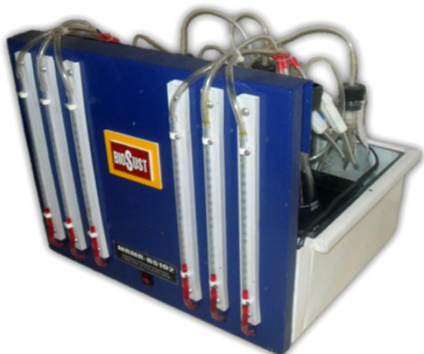
Fig. 2 The BMRS with six measuring units at the front side and the reaction section (partially shown) at the rear side
