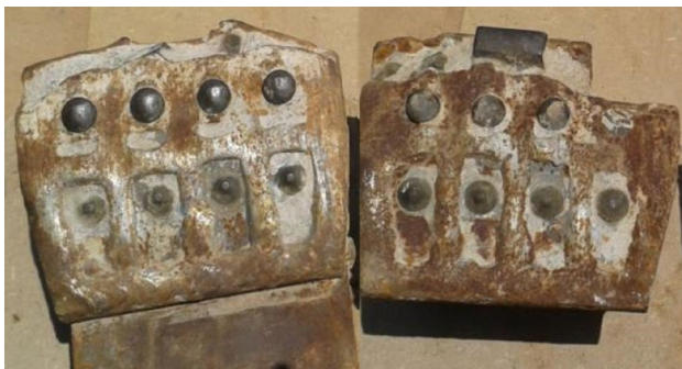
Fig. 2 Samples of worn scrapers in the case study tunnel
