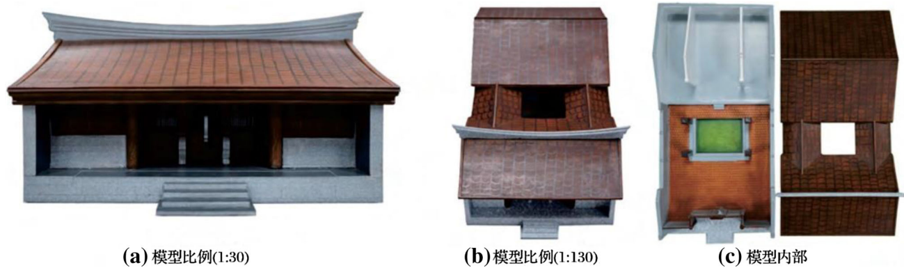
Fig. 10 Printing model 3D ancient building
