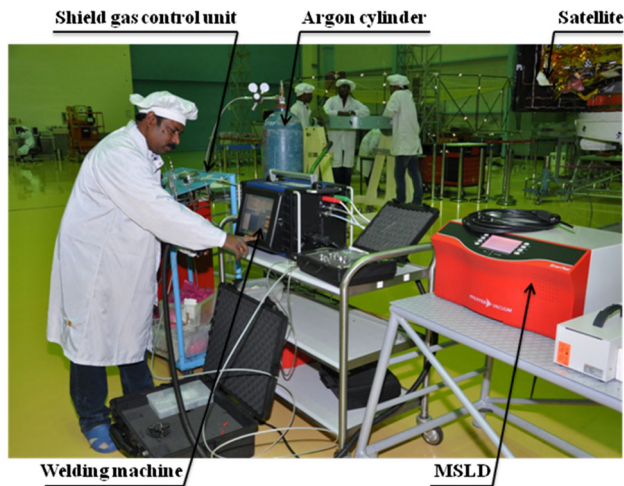
Fig. 4 Orbital TIG welding experimental setup
