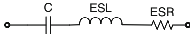
Fig. 5 Simplified model of an aluminum electrolytic capacitor equivalent circuit (Application guide, Cornell Dubilier), under normal operation
