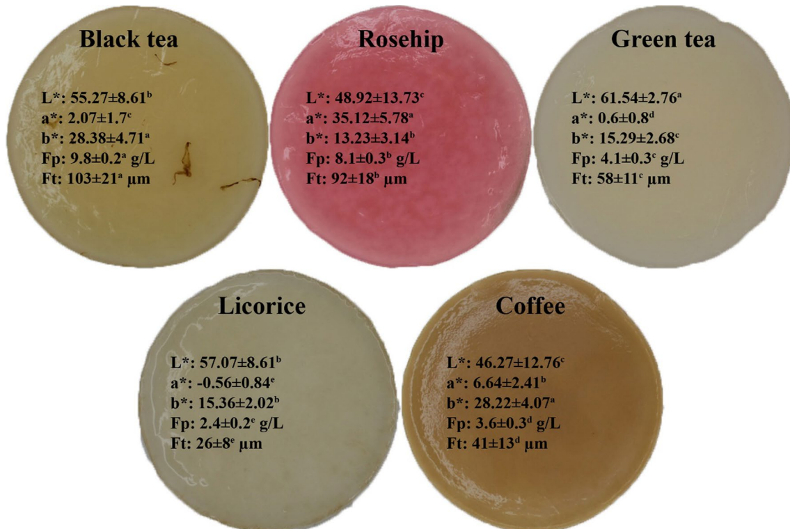
Fig. 2 Native films and physical properties of plant infusions. L^* : darkness-lightness, a^* : redness-greenness, b^* : yellowness/blueness, Fp: film productivity, Ft: film thickness. Significant differences ( p < 0.05 ) between the properties of the samples are indicated by different letters
