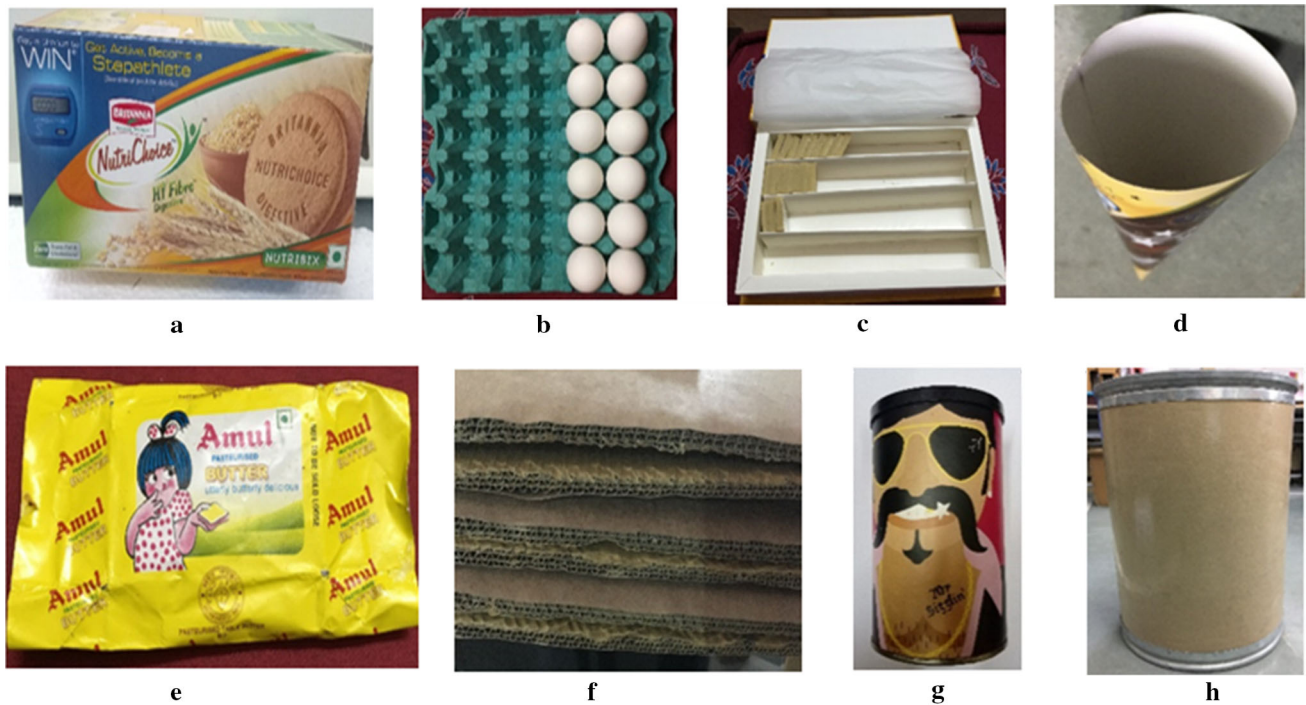
Fig. 2 Paper and paperboard based packaging materials used for food packaging application, a biscuits packed in paper based boxes, b egg crates, an example of moulded pulp packaging material, c paperboard
