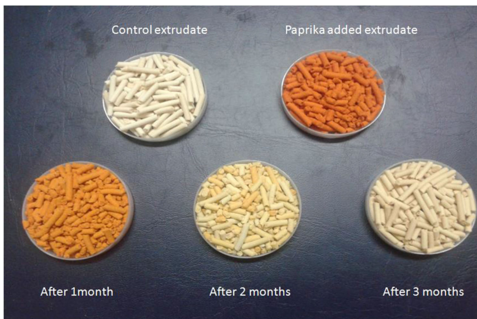
Fig. 1 Photographic images of control (without addition of paprika) and optimized rice:paprika blend extrudate (packed in vacuum packaging, stored at 25 °C with 65 % relative humidity) as a function of storage time indicating colour degradation
