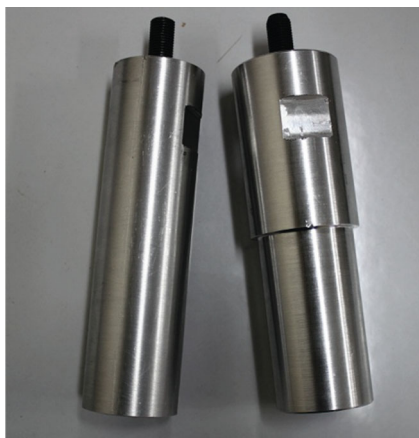
Fig. 7 End view of the produced horns (step horn on the right and cylinder horn on the left)
