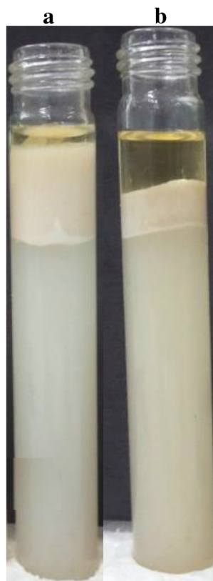
Fig. 8 Application of the extracellular pectinases produced by B. mojavensis I4 in the improvement of sesame seeds oil extraction. a: Test without enzyme, b: test with enzyme
