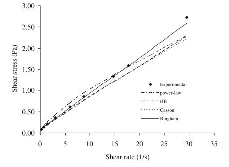
Fig. 4 The shear rate /shear stress data obtained from forward and backward directions of salep milk mixtures at 50 °C
