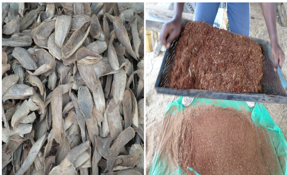
Fig. 2 Preparation of Coconut Fibres for the Study; a = Dried Coconut husk, b = Sieving of milled Coconut husks, and sawdust to obtain mixed sized of the fibres
