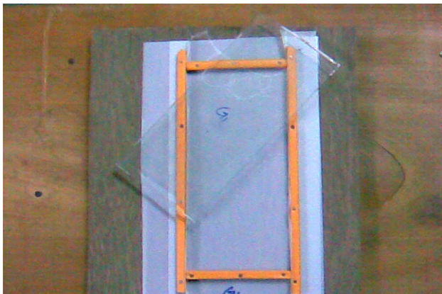
Fig. 2 Wooden mold for fabrication of composite
