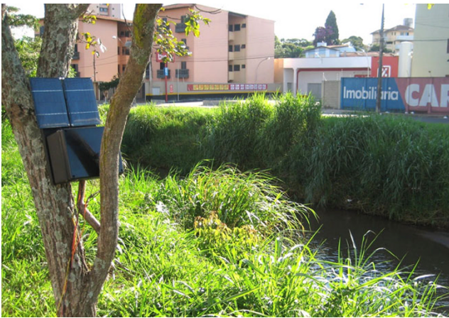
Fig. 10 A REDE sensor node being tested at the deployment site
