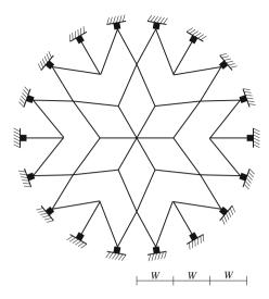
same as in (36), being a linear function of  $\eta$ . Each member of the frame is assumed to have a circular solid cross-section with radius  $r_j$ . Then we have  $\eta_j = \pi r_j^2$  and  $\xi_j = \frac{1}{4}\pi r_j^4$ .
